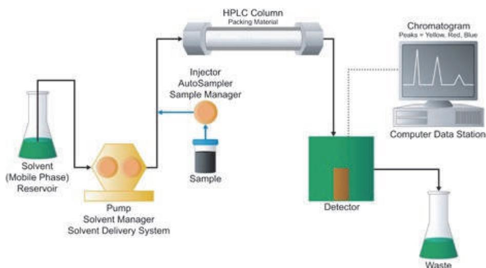
**Fig.46. HPLC Instrumentation**
