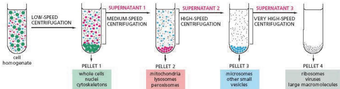
**Fig.26.2. Differential Centrifugation**
