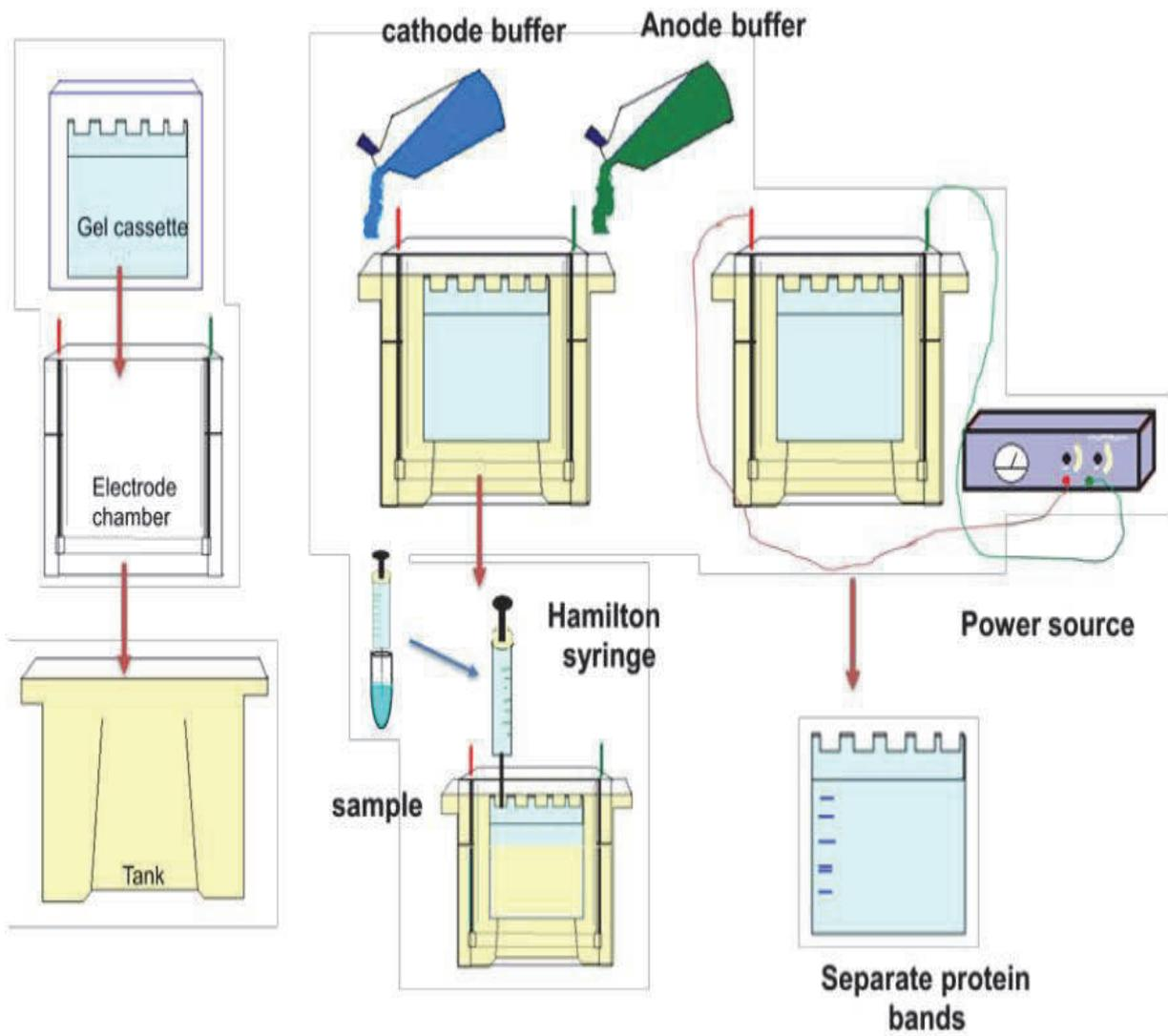
Fig.34.1 Casting of the Gel
