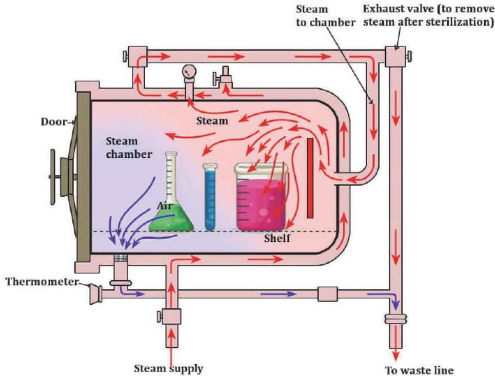
**Fig.24.1. Principle of Autoclave**
