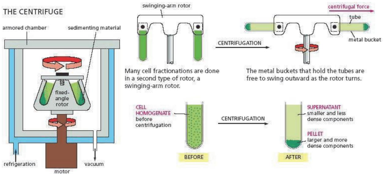
**Fig.26.1. Rotors and Centrifugation**
