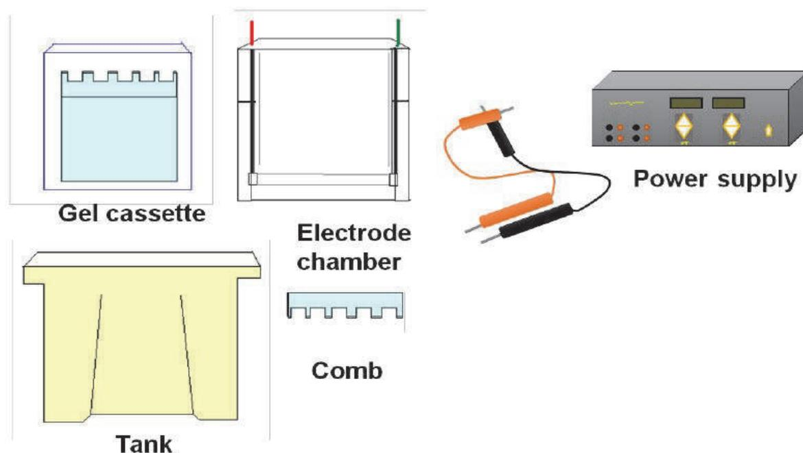
Fig.34. SDS-PAGE Instrument
