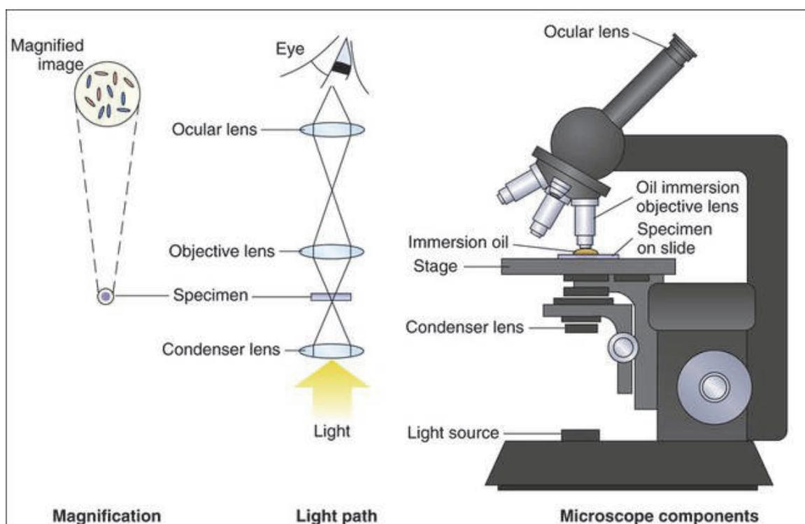
Fig.18.1. Working Principle of a Microscope
