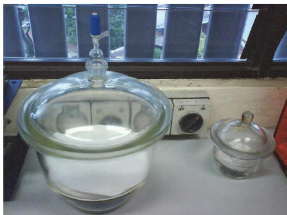
**Fig.7. Vacuum desiccators(left) & Desiccators (right)**
