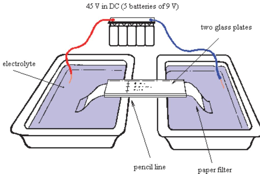
**Fig.33. Paper electrophoresis**
