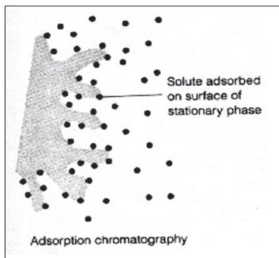
**Fig.35. Adsorption Chromatography**
